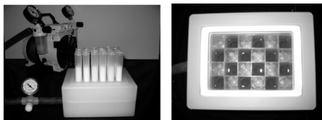
Figure 1. Plate-to-plate SPE system: (A, left) a 4 \times 6 VacMaster system connecting to a Wob-L piston vacuum pump and (B, right) 10-mL receiving well containing blue dye for cross-contamination test.
